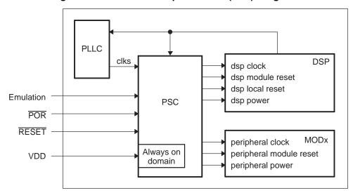
Figure 6-1. Power and Sleep Controller (PSC) Integration
